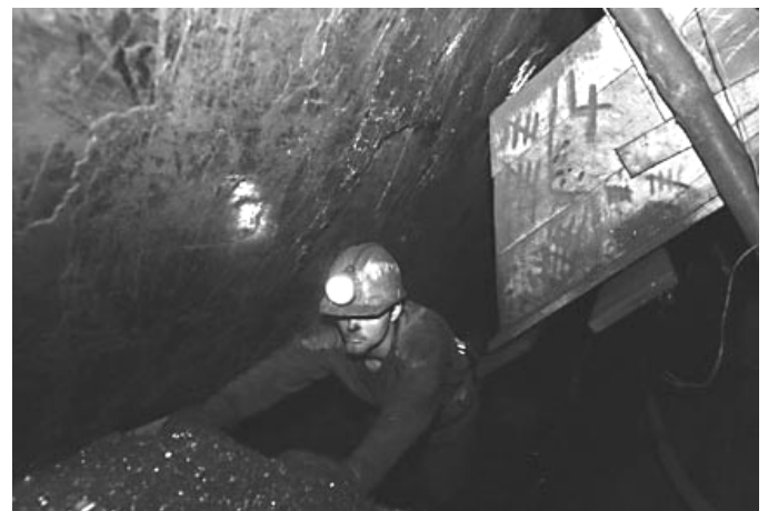
Steve Shingara pushes anthracite through the gangway, toward the buggy. The markings on the chute indicate how many buggies of coal were filled from that chute.
