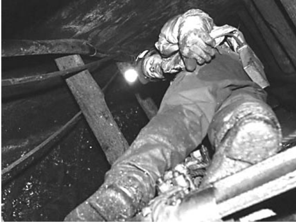
Tom rides on a narrow bar across the top of the buggy. When ice freezes along the chute, the miners sometimes need to force the buggy while standing on the bar to avoid getting stuck.
